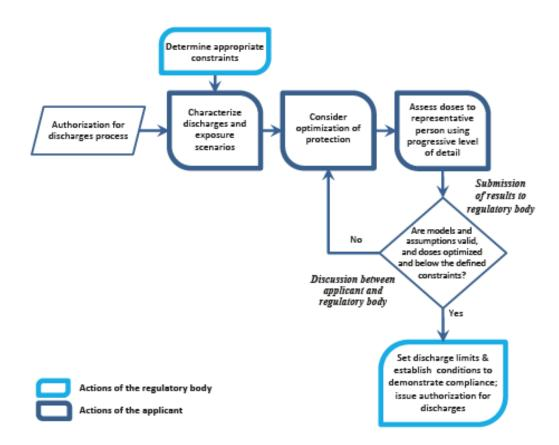
Fig. II-2: Steps in setting discharge limits, indicating those responsible (fig. 3 of GSG-9 [5]).
