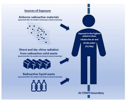
Fig. II-1: Illustration of the concept of the dose criterion for a hypothetical person at the FDNPS boundary.
